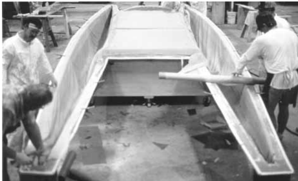
Figure 4-4 After applying an inner layer of fiberglass cloth, release fabric is placed over the laminates.
